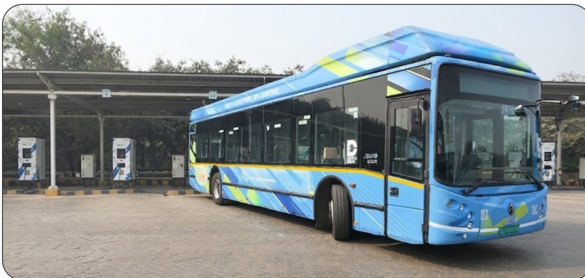
→ Buses charging at depot facility, Delhi Transport Corporation, ©UITP India
